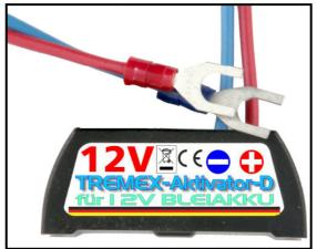
ly cause the detachment of the plaque and thus a decrease in sulfation. These pulses are measured in time so short that the load on the battery is very low. The effect is low internal resistance and thus a significantly higher capacity of the battery
